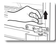
1. Separate the Cap on the Middle Hinge.
